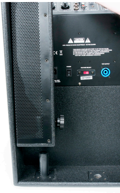
When the screw is loose enough, remove the array speaker from the base.
