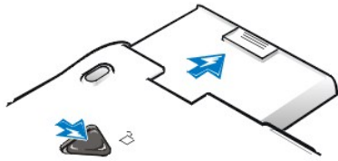
Figure 2. Installing a Battery
