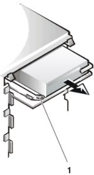
Figure 11. Removing a Diskette Drive From a Drive Bay
