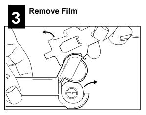
• Use tool to bend cover back and remove film.
