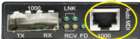
Auto MDI marked next to the RJ-45 port on the front panel of Model 515386.
