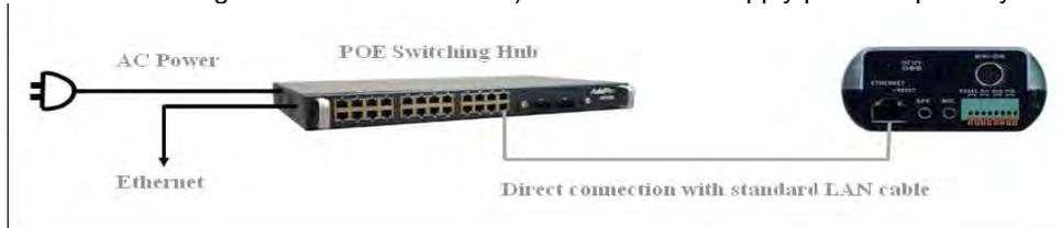
The standard IEEE 802.3af describes two types of devices: Power Sourcing Equipment (PSE) and Powered Devices (PD). Power sourcing equipment provides power to the powered devices. The network camera represents the powered device, whereas a PoE Injector is a PSE device. The Pro Series Network Camera models, *except* for model 550710, are IEEE 802.3af standard PoE compliant. They can be used with any IEEE 802.3af-compliant PoE injector.
