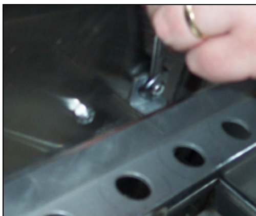
Removing the bracket nut
