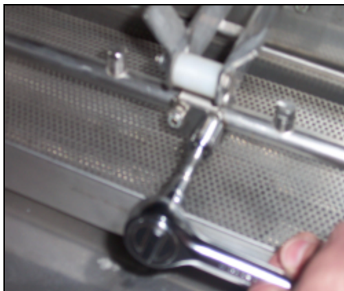
Removing the lower rinse arm support bracket
