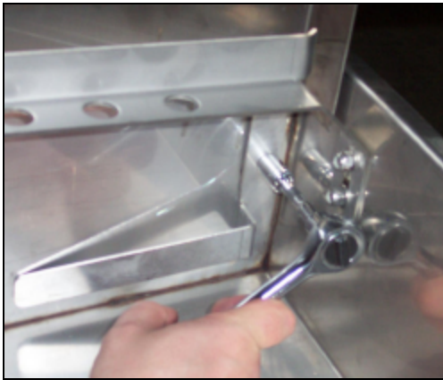
Removing a rinse tray guide bracket
