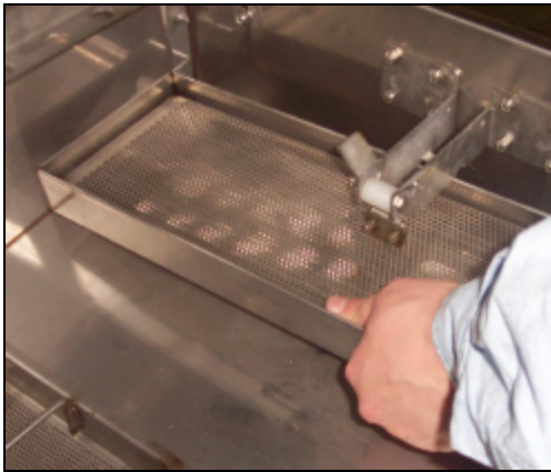
Lifting out the rinse tray assembly
