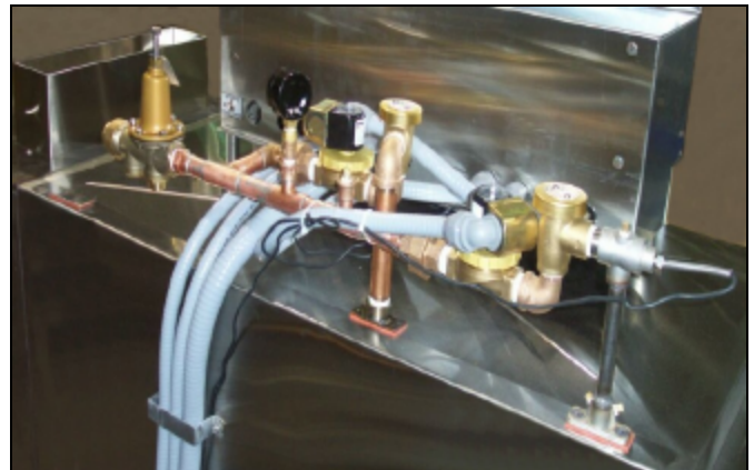
Incoming plumbing assembly for a Right to Left machine (note hole cover weldment in upper left corner)
