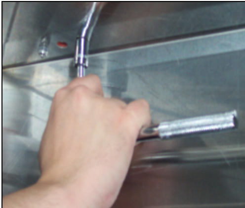
Removing the hole cover weldment
