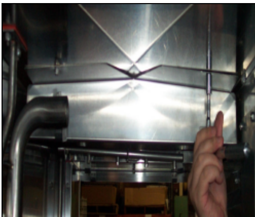
Removing and turning splash shield
