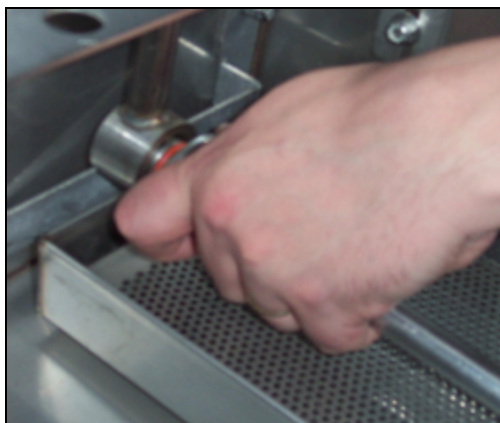
Unscrewing and removing the lower rinse arm
