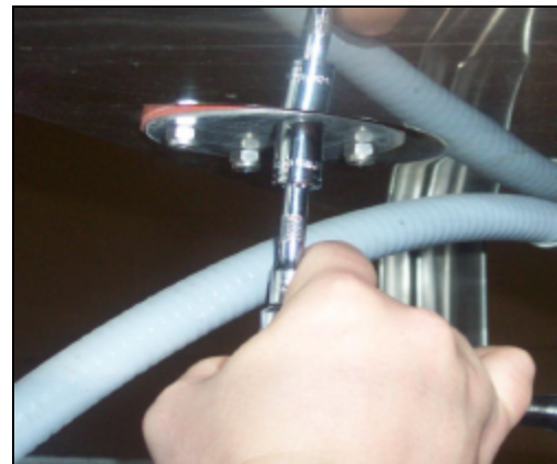
Removing the rinse drain plug
