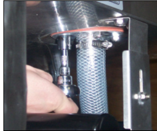
Removing the rinse drain weldment
