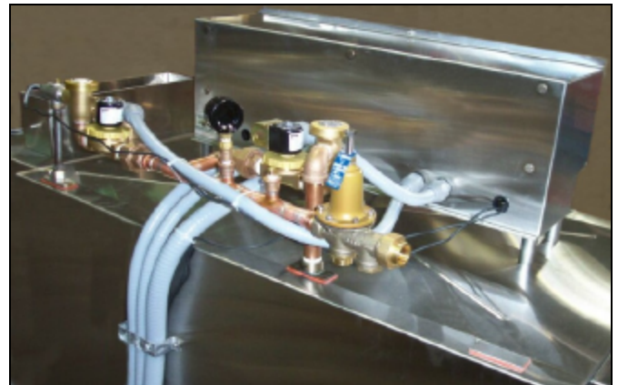
Incoming plumbing assembly for a Left to Right machine (note hole cover weldment in lower right corner)
