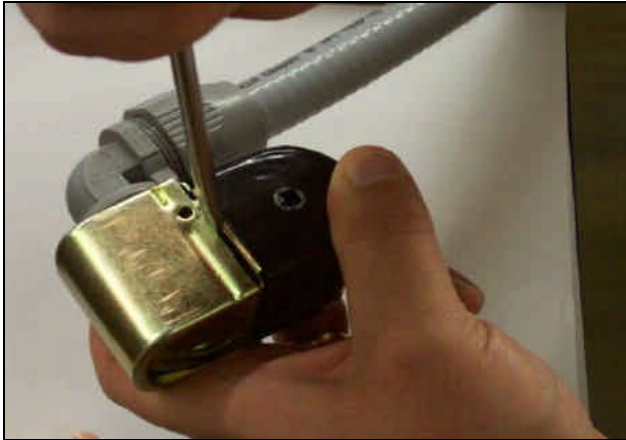
Prying open the coil wire cover
