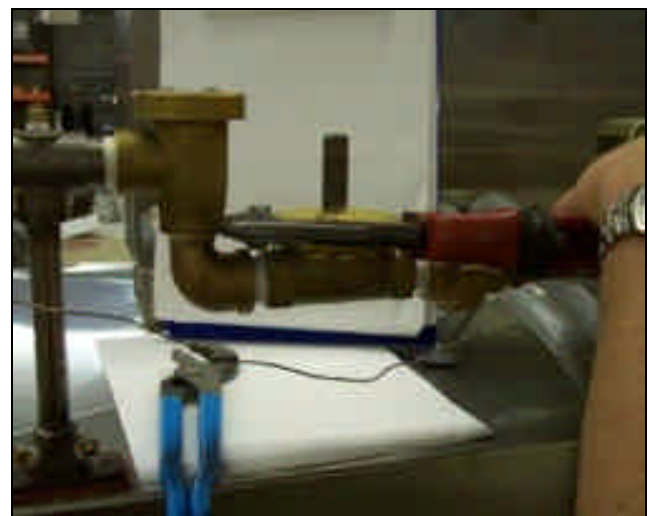
Loosening the valve bonnet
