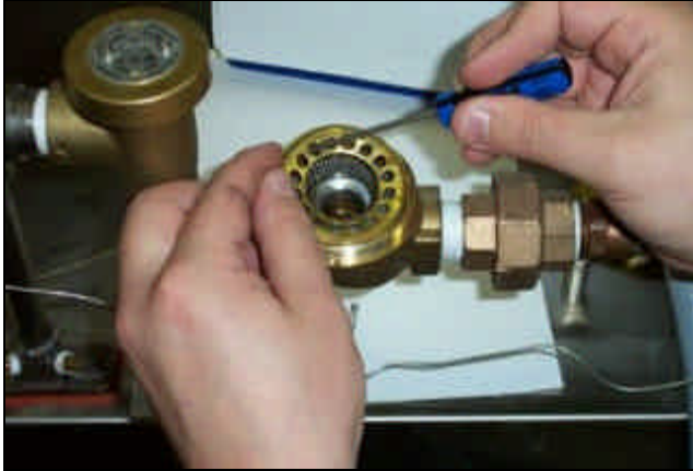
Removing the screen retainer
