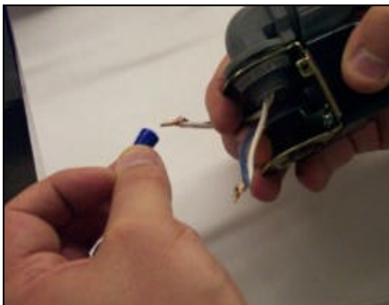
Removing the wire nuts
