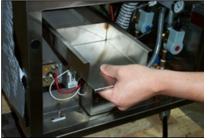
Removing upper (wash) strainer.
