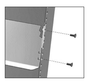
4. Slide the unit into the cabinet and secure it to the cabinet with a single #10-32 screw on each side.
