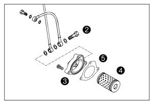
Place the new oil filter **4** on the connection in the oil filter cover and mount together with a new seal **5**. Tighten the 3 screws in the filter cover to 5 Nm (4 ft.lb). Tighten the hollow screw with seals and tighten to 15 Nm. Finally, start the engine and check the oil system for leakage.
