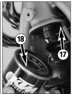
The screw  $\ensuremath{\mathbf{0}}$  must be removed to allow the motor oil to flow out of the frame breast pipe.
