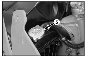
Pressure induced by heating of the cooling liquid in the cooling system is controlled by a valve in the radiator cap 6; a water temperature rising up to 120° C (248° F) is admissible, without fear of problems.
