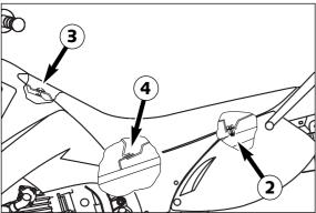
To mount the seat hook it into the oval head screw, lower the rear part of the seat and push the whole seat forwards. If necessary push the middle of the seat slightly down to let the retaining bracket ④ engage with the seat. Finally fasten the seat with the corresponding screw.
