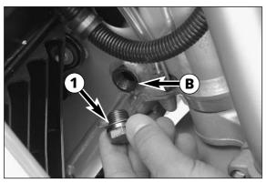
Fill 0.6 liters of engine oil into the can and remove the plug ① next to the steering head. Introduce the plastic hose into the vent hole ③, (see page 30) and fill 0.6 liters of engine oil into the frame's front tube. Remove plastic hose, start engine, and let it idle (approx. 20 seconds) until oil escapes at the hole ⑤. As soon as oil starts to escape, turn off the engine, and mount the plug together with the gasket.
