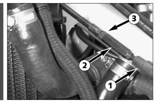
Push the choke lever all the way to the front and slide the protecting cap from the adjusting part ②.
