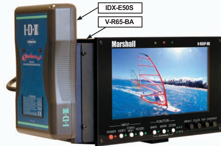
V-R65P-HD shown with V-LCD4-MT camera hot shoe mount attached plus rear mount configuration of V-R65-BA adaptor and IDX-E50S battery
