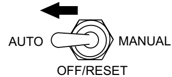
Figure 36. MPEC Control Switch (AUTO)
