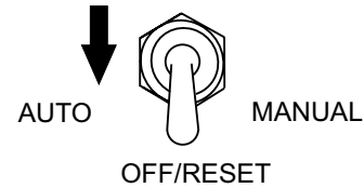
Figure 38. MPEC Control Switch (Off/Reset)
