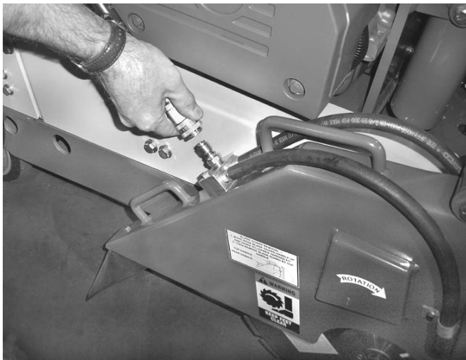
Figure 15. Blade Guard Water Delivery Connector
