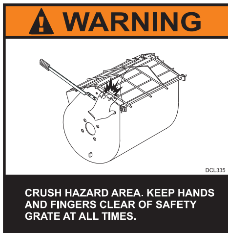
Figure 42. Safety Grate (Crush Hazard)
