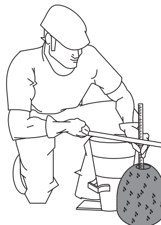
Figure 41-F. Slump Test (Measurement)
