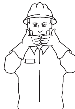
ALL DONE CLEAN-UP
