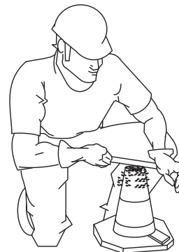
Figure 34-D. Slump Test (Removing Excess Concrete)
