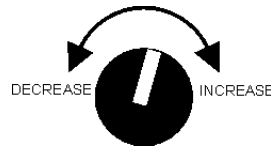
FIGURE 37. Voltage Regulator Knob located on the control panel
