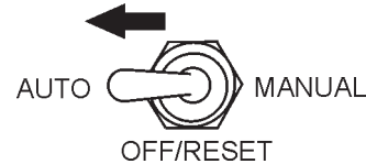
Figure 41. MPEC Control Switch (AUTO)
