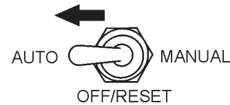
Figure 55. MPEC Control Switch (AUTO)
