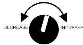
FIGURE 36. Voltage Regulator Knob located on the control panel
