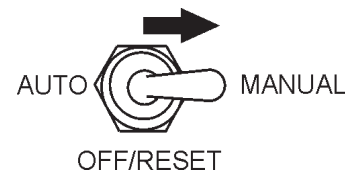
Figure 42. MPEC Control Switch (Manual Position)
