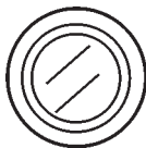
Figure 41. Main Circuit Breaker OFF Lamp
