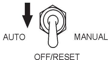
Figure 66. MPEC Control Switch (Off/Reset)
