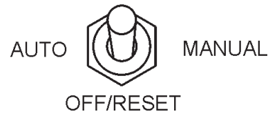
Figure 74. Off/Manual Auto Switch (Off)
