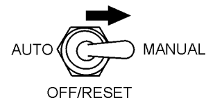
Figure 41. MPEC Control Switch (Manual Position)
