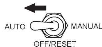
Figure 54. MPEC Control Switch (AUTO)
