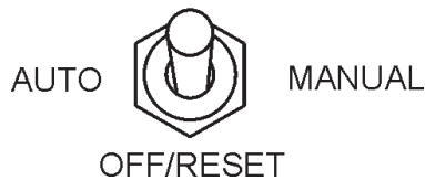
Figure 55. MPEC Control Switch (Off/Reset)
