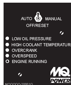
Figure 41. MPEC Engine Running Status LED
