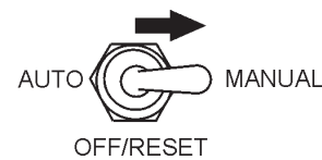
Figure 39. MPEC Control Switch (Manual Position)
