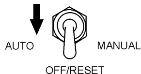
Figure 54. MPEC Control Switch (Off/Reset)
