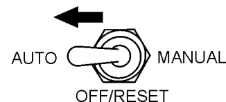
Figure 52. MPEC Control Switch (AUTO)
