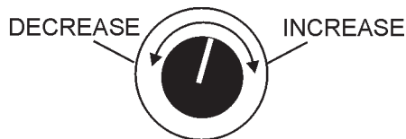
Figure 44. Voltage Adjust Control Knob
