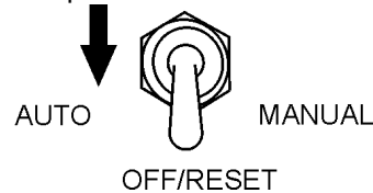
Figure 55. MPEC Control Switch (Off/Reset)
