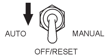
Figure 58. MPEC Control Switch (Off/Reset)
