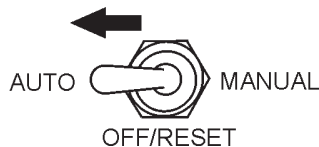
Figure 55. MPEC Control Switch (AUTO)
