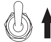
Figure 13. Operation Switch (ON Position)
