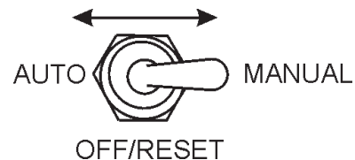
Figure 44. MPEC Control Switch (Manual Position)
