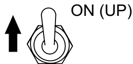
Figure 18. Control Power Switch (ON)
