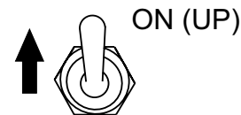
Figure 22. Fuel Priming Switch (ON)
