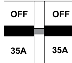
Figure 25. Main Circuit Breaker (OFF)
