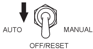
Figure 54. MPEC Control Switch (Off/Reset)
