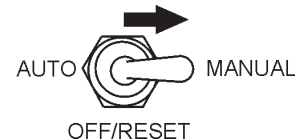
Figure 38. MPEC Control Switch (Manual Position)
