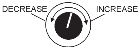
Figure 20. Voltage Regulator Knob
