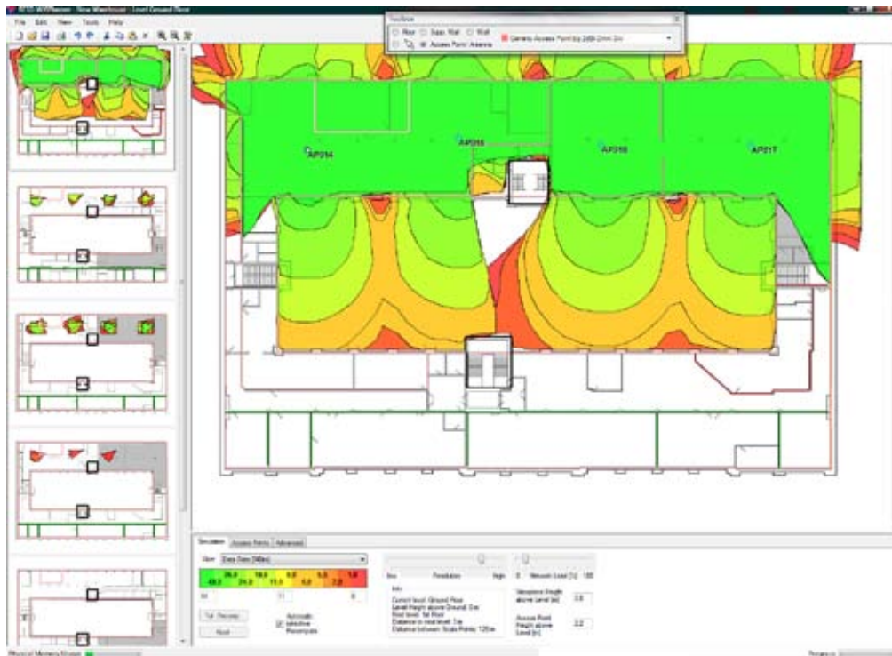
Checking the results of access point settings in the Data Rate view.
