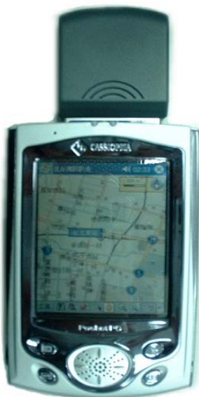
Image 1: TN202 installed in PDA
