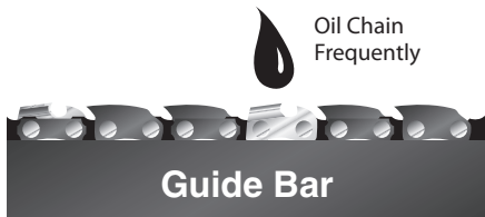
Figure 12 - Applying Oil to Chain
