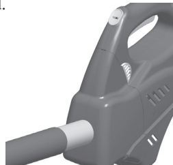
Figure 25 - Assembled Main Handle and Handle Adapter
