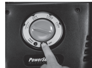
Figure 20 - Press Circuit Breaker
