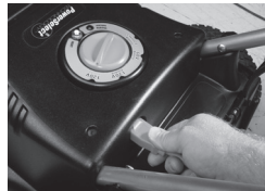
Figure 15 - Plugging Extension Cord
