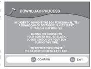
**Note:** if the download process is not correctly performed, the screen stays black and the green led flashes indicating the cause of the failure (see table below).
