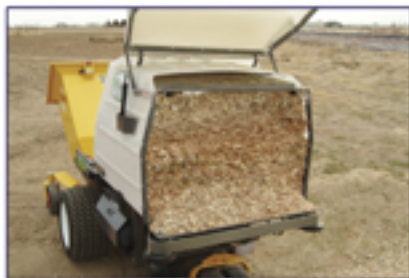
Catcher box fills completely with chipped material
