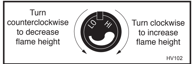
Fig. 23 Flame adjustment knob for Honeywell Valve.
