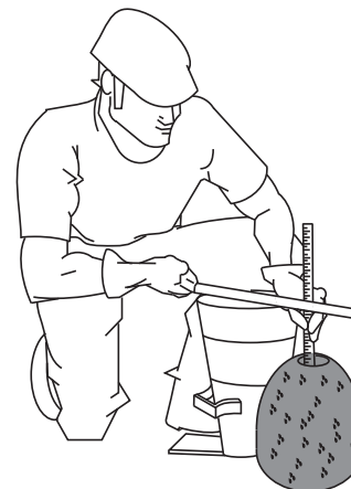
Figure 41-F. Slump Test (Measurement)
