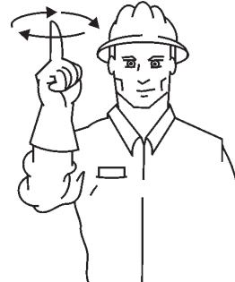
START PUMP SPEED UP
