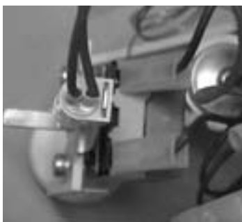
Thermostat spade connectors
