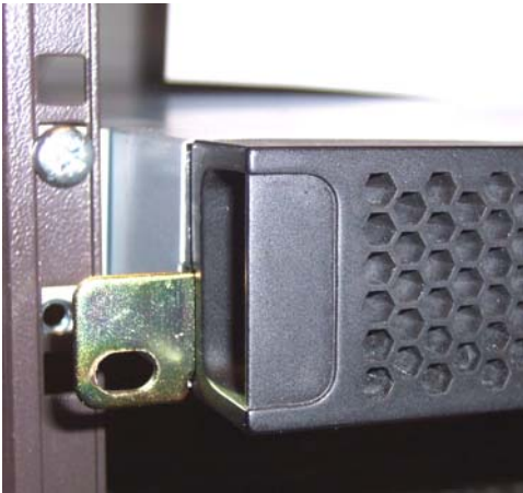
Figure 6. Slide the FastStor 1 in from the front.
