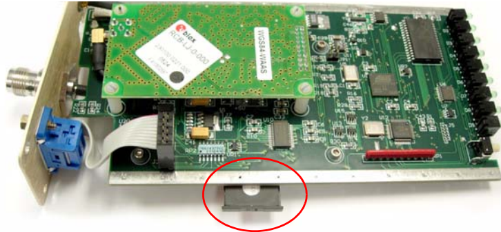
FIGURE 5. Inserting the SIM: PinPoint
