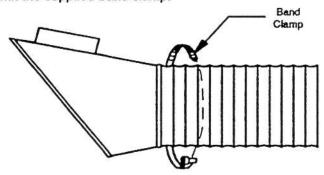
Mount the hose assembly to the unit. Using the cotter pin supplied, attach the shaft of the hose swivel from inside the unit.
